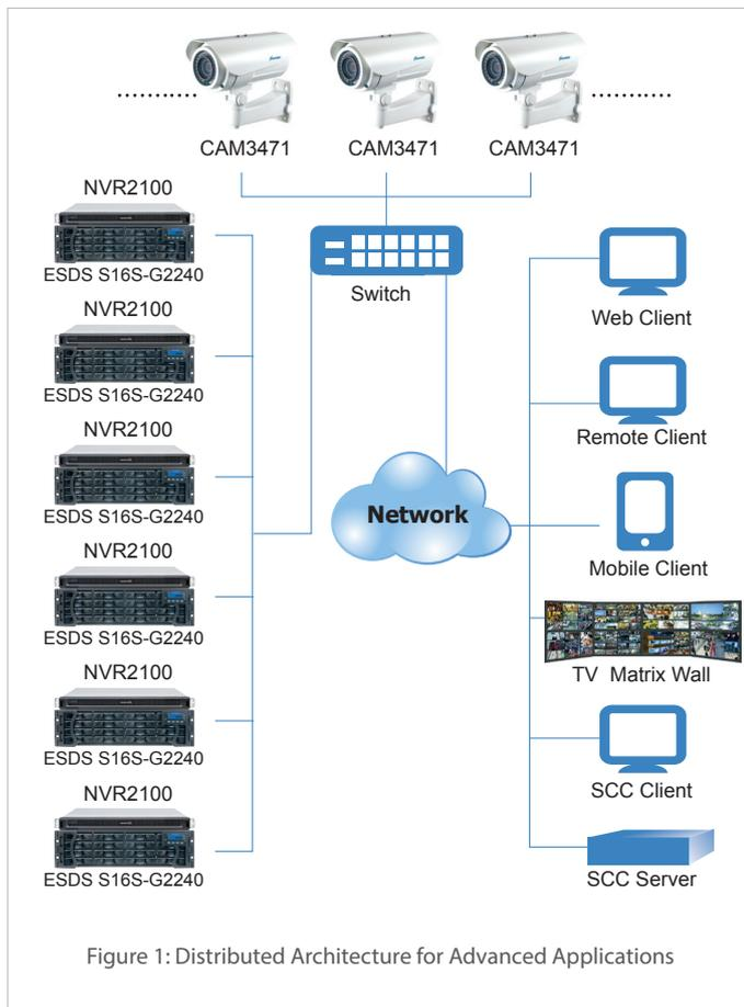
Figure 1: Distributed Architecture for Advanced Applications
