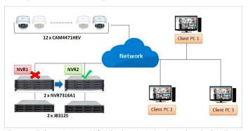
Figure 3: Failover Activated (If NVR1 down) – Video Records to Both NVR2 & NVR2's JBOD
