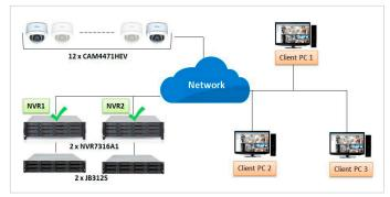
Figure 2: Normal Recording - Video Records to Both NVR1 & NVR2
