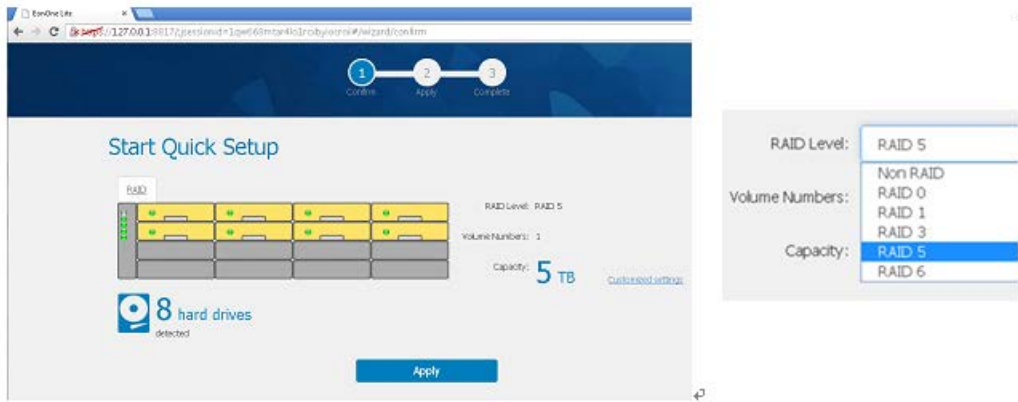
(3-step setup wizard for fast and easy RAID storage setup and can begin monitoring system statuses)
