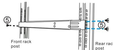
2-6. To fix the slide rails' length, attach a bracket support (04) to slide rail using three M5 x L10 crosshead screws (06).
