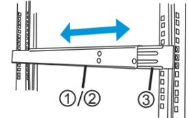
2-5. Screw one M5 x 5mm position screw (05) to the front rack post and two M5 x 5mm position screws (05) to the rear rack post (top and bottom positions) to secure the slide rail to the rack.
