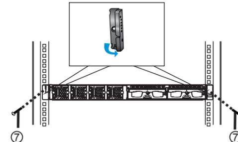
2-9. Secure the panel back onto the enclosure to complete the rack mount procedure.
