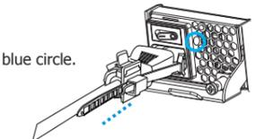
5-5. Flip power buttons to the ON position on BOTH PSUs.
