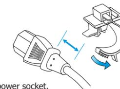
5-3. Connect the power cord to the power socket.
