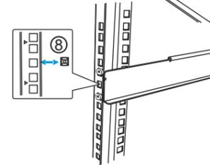
2-8. Lift the enclosure and align it with the slide rails on the rack, keeping pressure even on both sides, slowly push the enclosure into the rack. Fasten one M5 x 35mm crosshead screw (07) on each side of the enclosure chassis ears to secure the enclosure onto the rack.
