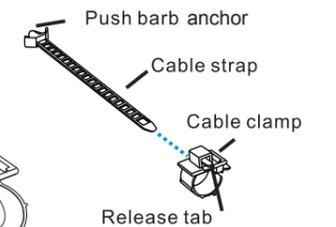
5-2. Wrap the cable clamp around the base of the power plug.
