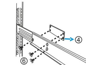
2-7. Attach one cage nut (08) to the front of the rack post. The cage nut will be used to secure the enclosure in place.
