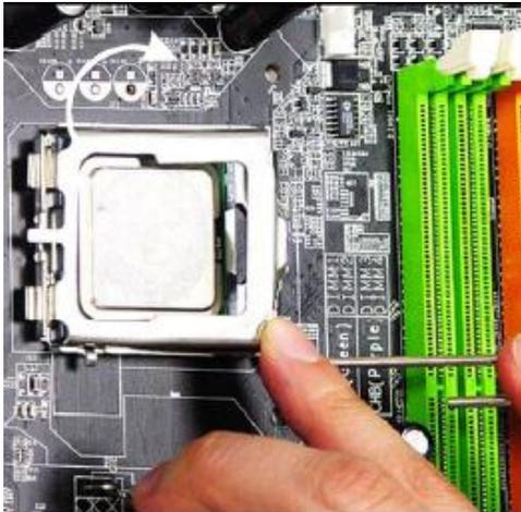
**Figure 3-4: Opening CPU Retention Cover**
