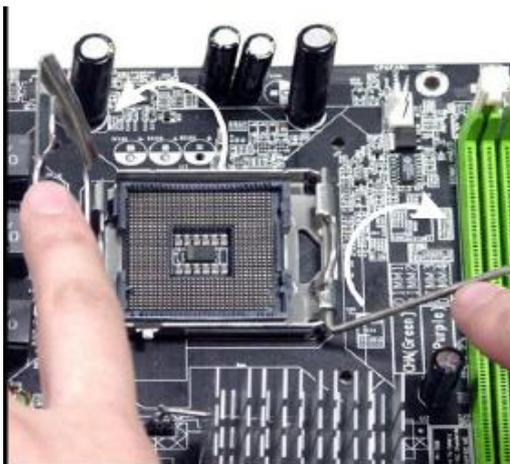
**Figure 3-5: CPU Socket**
