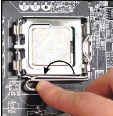
**Figure 3-3: Opening CPU Retention Cover**
