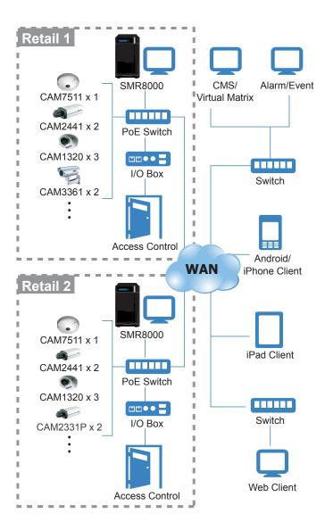
Figure 1: Distributed Architecture for Advanced Applications
