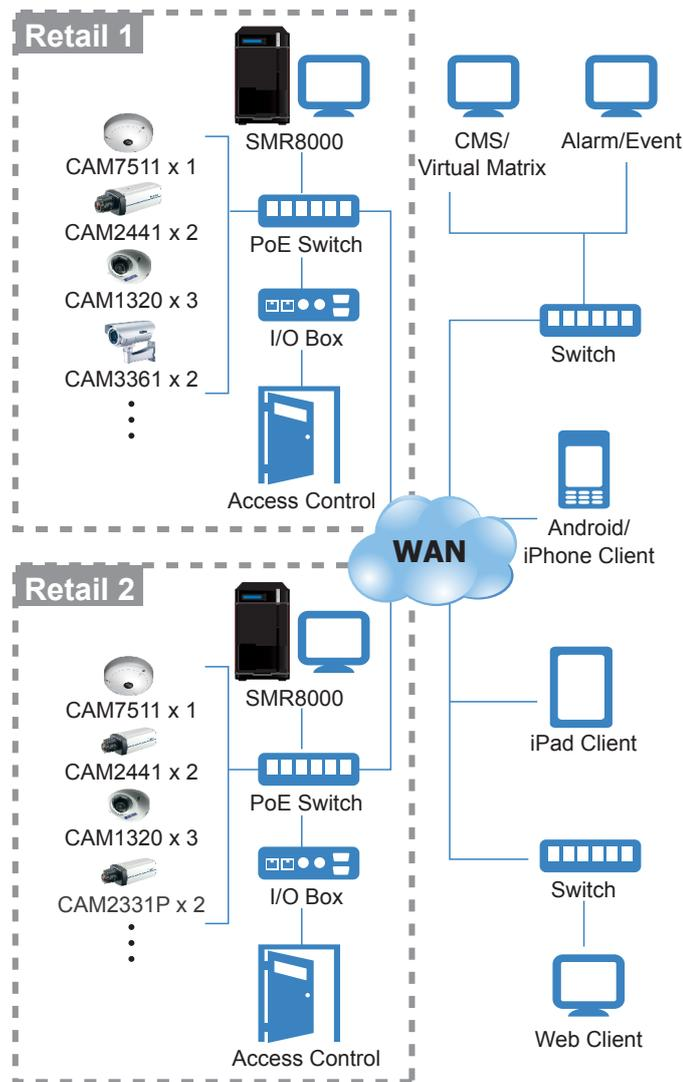
Figure 1: Distributed Architecture for Advanced Applications
