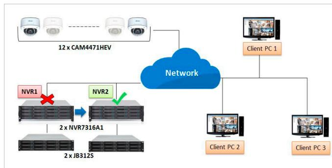
Figure 3: Failover Activated (If NVR1 down) – Video Records to Both NVR2 & NVR2's JBOD
