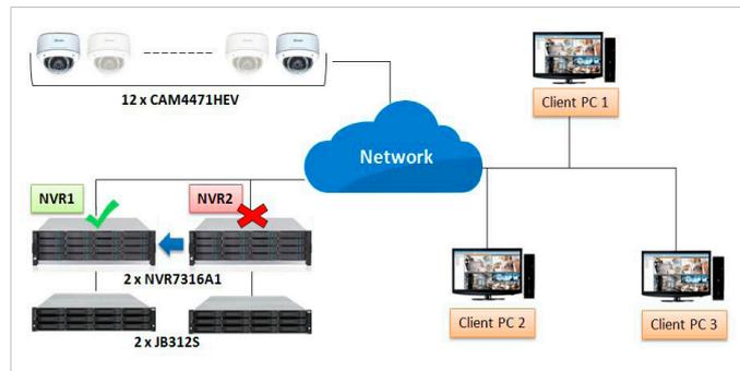
Figure 4: Failover Activated (If NVR2 down) – Video Records to Both NVR1 & NVR1's JBOD
