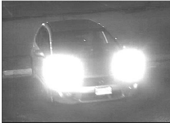
Cameras can't figure out how to expose the image properly.
