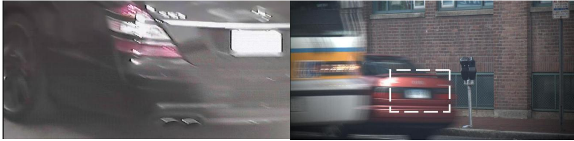
Typical examples of the side to side motion blur.
