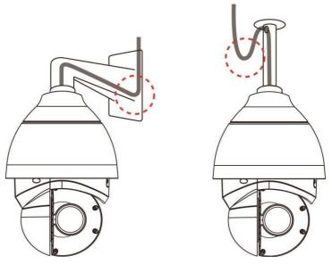
• The cable entry hole of the outdoor mounting kit (indicated in the figure below) needs to be sealed with thread seal tape to avoid water from entering the camera.
