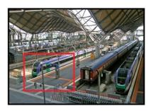
Users can configure up to 10 sets of Motion Detection Windows in each set of Motion Detection Setting. Click on the <add> button under the Live Video Pane to add a Motion Detection Window. To cancel a Motion Detection Window, move the mouse cursor to the selected Window, and click on the <delete> button.
