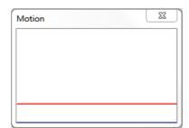
When motion is detected, the signals will be displayed on the Motion window as shown below. Motion is detected by comparing sampling pixels in the detection area of two consecutive live images.
