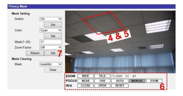
**Step 4.** To shift the mask to the intended location, move the mouse cursor to the center of the mask and click and drag.
